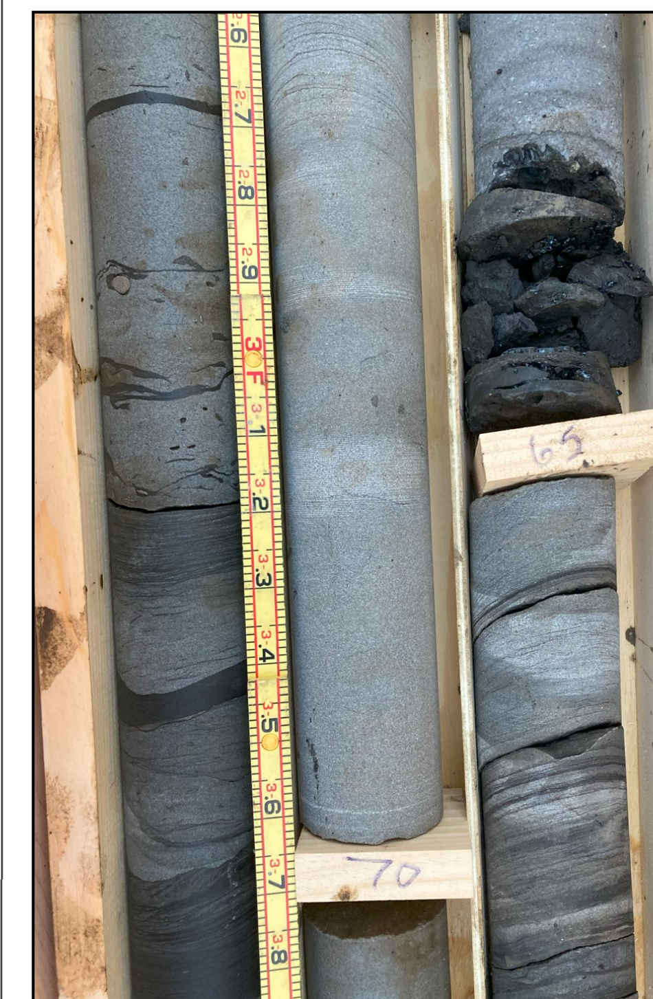
Major fracture and coal seam at 65' bgs, where artesian flow left the borehole.
