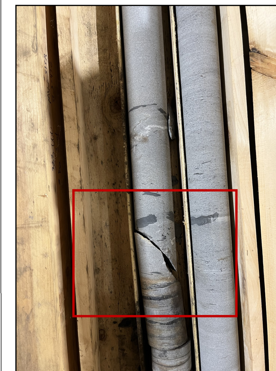
Major fracture in Deep Aquifer sandstone at 158' bgs, where artesian flow entered the borehole.
