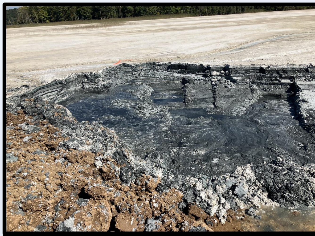
High water content observed near the impoundment surface.
