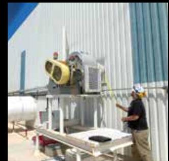
*TOP: As part of the air permit requirements, stack testing is performed at this lime plant in Ste. Genevieve, MO.*
